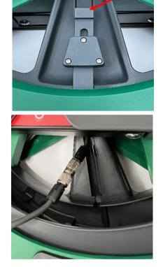
8. Replace the connector connection and cable in the space provided.
